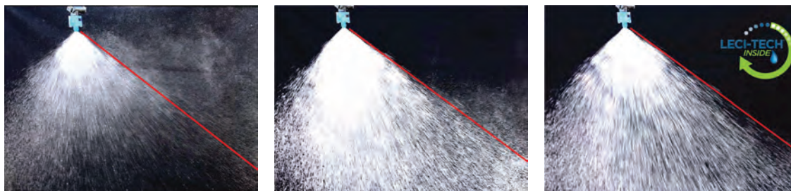
Demonstrates in simulated wind, coarse droplets of; water alone (left), water with glyphosate (middle), and water with glyphosate and Leci-Tech® (right).
